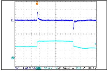
Figure 6: Output voltage response to step-change in input voltage (1V/ms). Load cap:  $1 \mu F$  ceramic capacitor. Ch 1: Vout, Ch 2: Vin.
