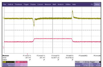
Figure 5: Output voltage response to step-change in load current (50%-75%-50% of lout(max);  $dVdt = 0.1~A/\mu s$ ). Load cap:  $1~\mu F$  ceramic and  $15~\mu F$  tantalum capacitors. Ch 1: Vout, Ch 2: lout (5A/div.)
