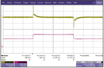
Figure 6: Output voltage response to step-change in input voltage (1V/ms). Load cap: 1 µF ceramic capacitor. Ch 1: Vout, Ch 2: Vin.
