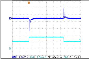
Figure 5: Output voltage response to step-change in load current (50%-75%-50% of Iout(max); dI/dt = 0.1 A/µs). Load cap: 1 µF ceramic capacitor. Ch 1: Vout, Ch 2: Iout (2.5A/div.)
