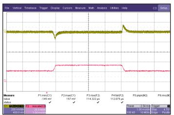
Figure 5: Output voltage response to step-change in load current (50%-75%-50% of lout(max);  $dI/dt = 0.1~A/\mu s$ ). Load cap: 1  $\mu F$  ceramic and 15  $\mu F$  tantalum capacitors. Ch 1: Vout, Ch 2: lout (10A/div.)
