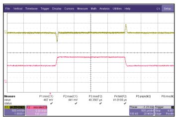
Figure 5: Output voltage response to step-change in load current (50%-75%-50% of lout(max);  $dI/dt = 0.1 \ A/\mu s$ ). Load cap:  $1 \ \mu F$  ceramic and  $15 \ \mu F$  tantalum capacitors. Ch 1: Vout, Ch 2: Iout (2.5 A/div).
