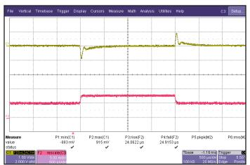
Figure 5: Output voltage response to step-change in load current (50%-75%-50% of lout(max);  $dI/dt = 0.1 \ A/\mu s$ ). Load cap:  $1 \ \mu F$  ceramic capacitor. Ch 1: Vout, Ch 2: lout (2.5A/div.)
