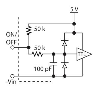
Figure B: Internal ON/OFF pin circuitry
